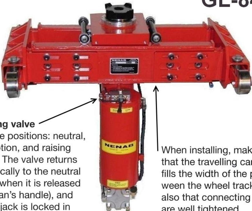
**Operating valve** with three positions: neutral, rapid motion, and raising position. The valve returns automatically to the neutral position when it is released (dead-man's handle), and then the jack is locked in the existing height position.
